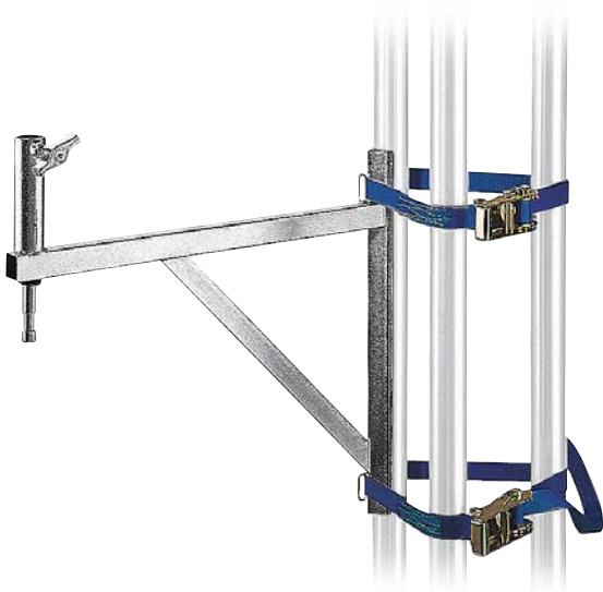
F1200 COLUMN ARM 3,1kg 6.8lb 10kg 22lb 16mm 5/8" 28mm 1" 1/8 Length: 51cm (20.1").
